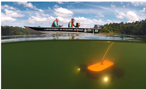
Fig. 2 Remotely operated vehicle model Genneino T1 being operated from a boat in the Lajes Reservoir, Rio de Janeiro State, Brazil
